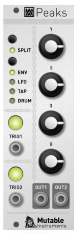
The **SPLIT** button toggles between the **twin** (LED off) and **split** (LED on) modes. Hold it for a second to enter the **expert** mode. In this mode, the button toggles between channel 1 and 2. Hold it for a second to get back to normal operation.
